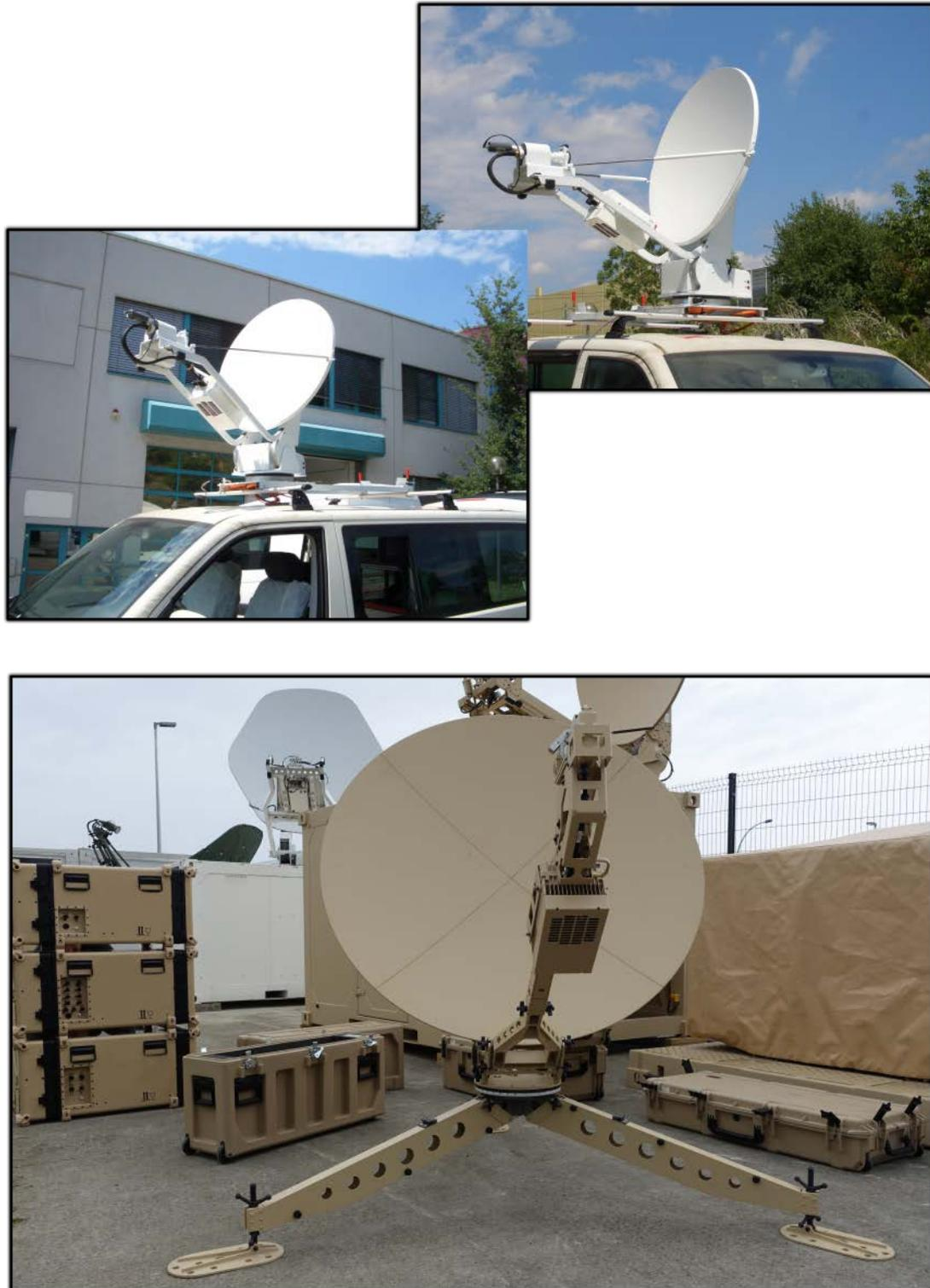
**Figure 3.3** IBUC 2 Installation
