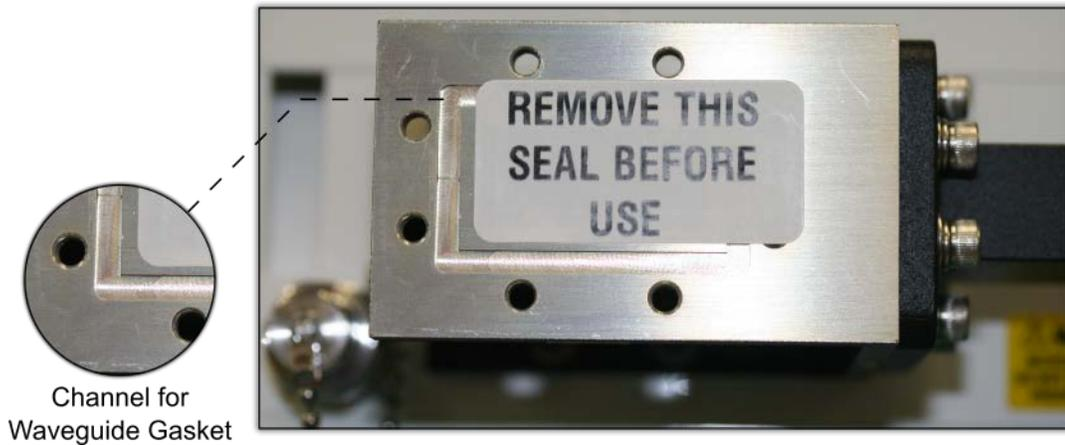
**Figure 3.9** Waveguide Label and Channel for Gasket
