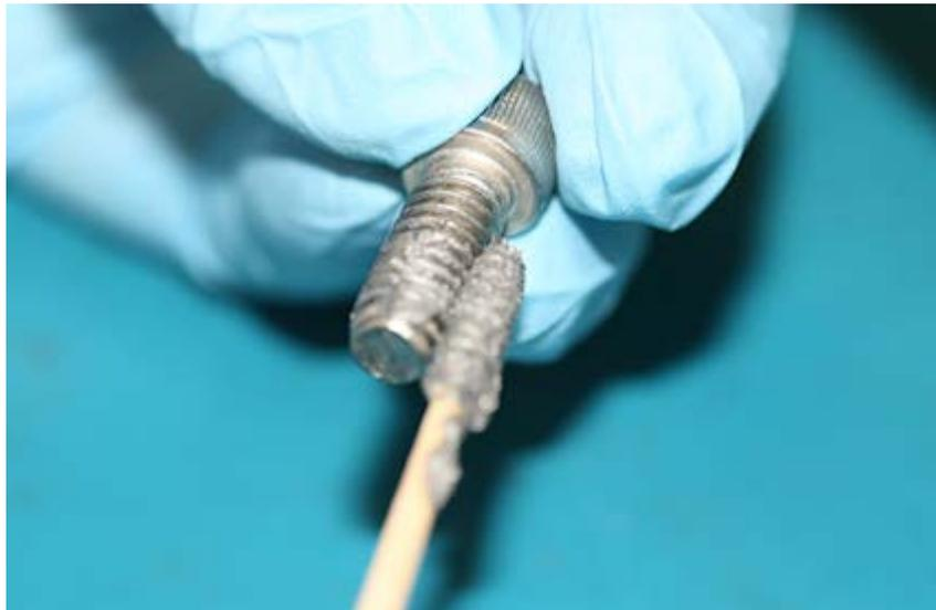
**Figure 3.8** Applying the Anti-Seize Lubricant
